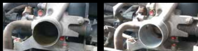
BEFORE (Throttle body condition after 60,000 km)
